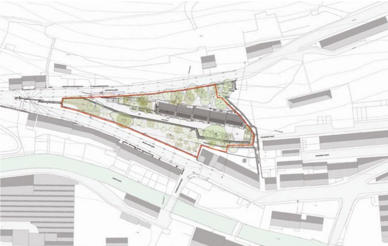
Proposed site plan showing the similarity of grain, reinstating housing to the High Street site at a lower density alongside retaining green amenity that the site has developed since the historical properties were demolished in the 1960s
